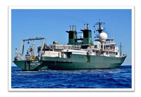
The globally capable 272-foot research vessel *Falkor* is Schmidt Ocean Institute's key operational asset. In 2012, SOI completed a full refitting of *Falkor*, an ice-strengthened former German fisheries vessel. She now has a 13,000-nautical-mile range and a max speed of 20 knots.
