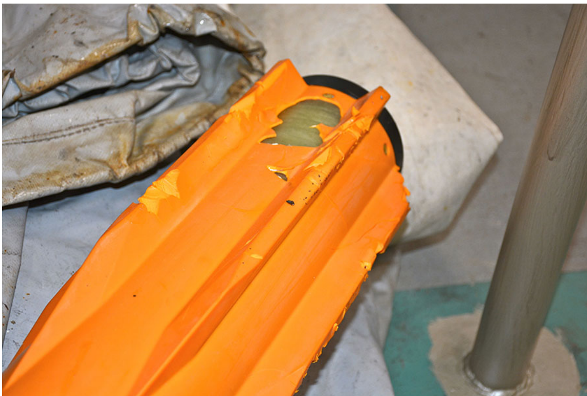
Figure 8. Damaged tail fins of the magnetometer.
