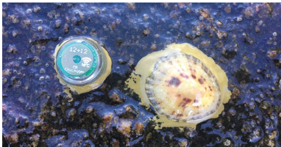
Naked and biomimicking ("Robo-limpet") temperature loggers attached to the rocks of the intertidal zone can measure substrate temperature at intervals of 10 seconds to 18 hours. Data is captured with an app and can be shared immediately providing that there is mobile coverage
