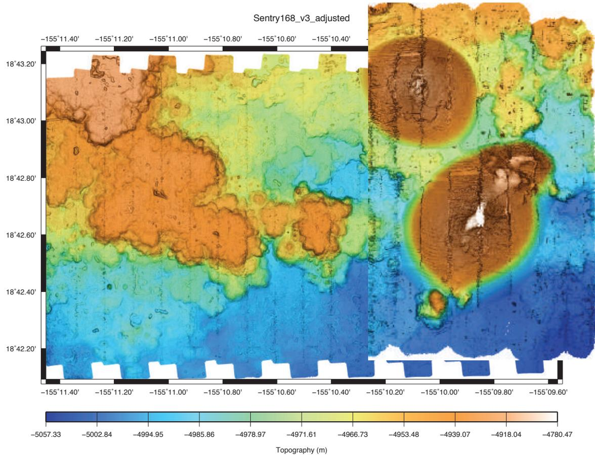
Figure 9 –Multibeam sonar bathymetry map of the FeMO Deep mats area and adjacent basalt features. Map is merged from three AUV *Sentry* dives, nav adjusted (*Sentry*-168 and *Sentry*-264, and *Sentry* 265).
