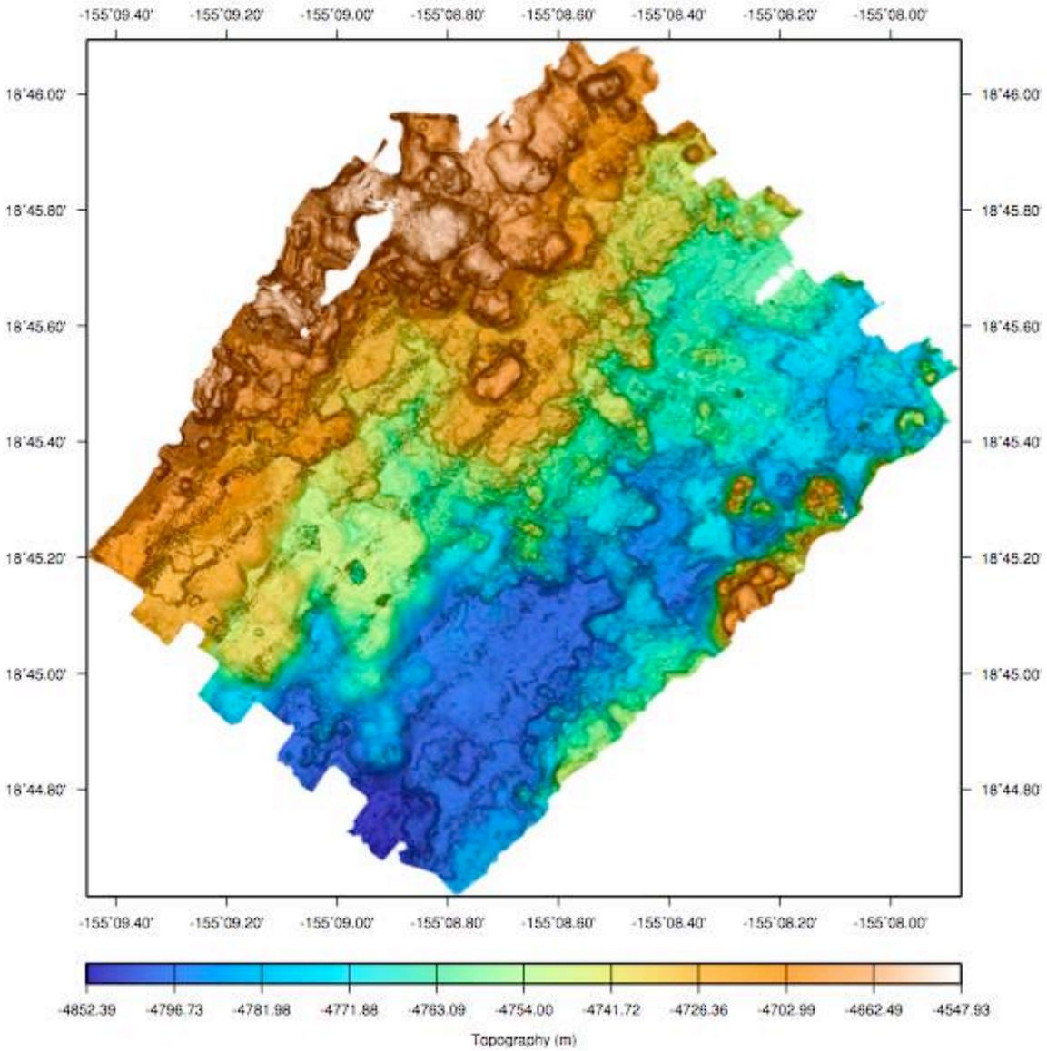
Figure 12 - Multibeam sonar bathymetry map of the basin and adjacent basalt features to the SW of Shinkai Deep. Map is a product of *Sentry-270*.
