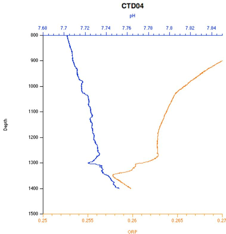
Figure 7 – pH and Oxidation-Reduction Potential (ORP) profiles collected on CTD Hydrocast 04 revealed anomalies associated with the dispersing hydrothermal plume at 1300m to 1350m, and informed specific depths to collect bottle samples on Casts-05, -06, -07.
