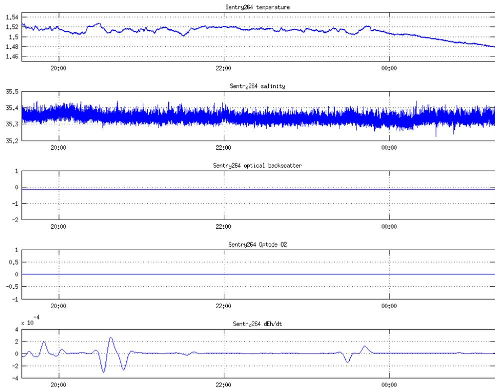
Figure 2: Time series plot of five of the basic sensors on Sentry, from top to bottom, temperature, salinity, optical backscatter, and dissolved Oxygen.
