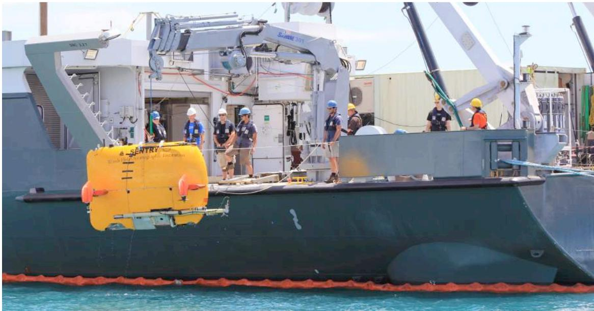
Figure 4 – Dockside testing of optimal launch and recovery procedures for AUV *Sentry* aboard R/V *Falkor* (photo credit: C. Wiener).
