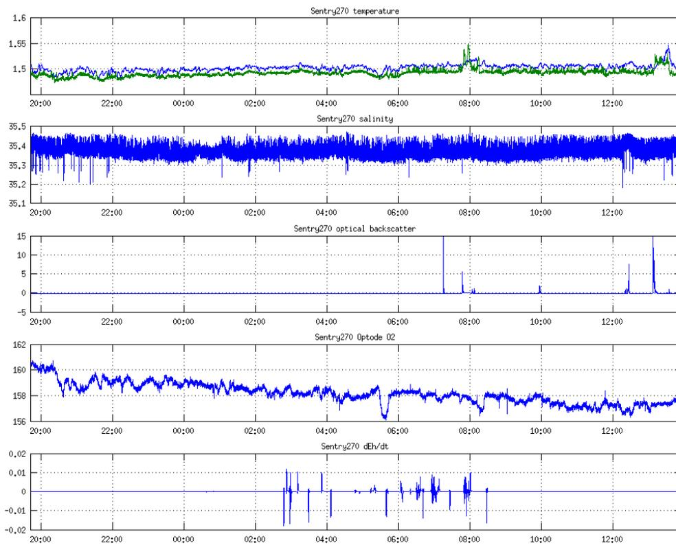
Figure 31: Time series plot of five of the basic sensors on Sentry, from top to bottom, temperature, salinity, optical backscatter, and dissolved Oxygen.
