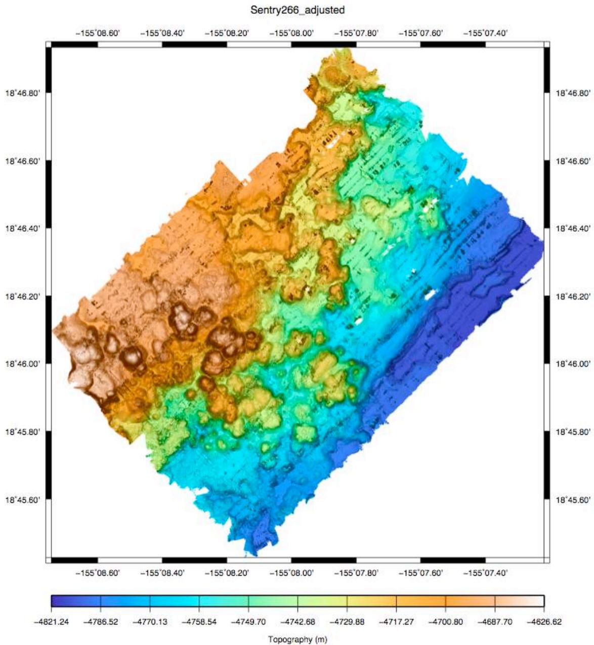
Figure 10 –Multibeam sonar bathymetry map of the Shinkai Deep area and adjacent basalt features. Map is a product of *Sentry*-266.
