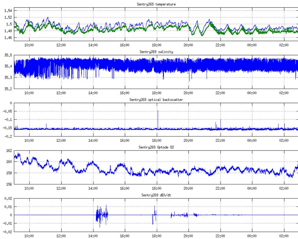
Figure 25: Time series plot of five of the basic sensors on Sentry, from top to bottom, temperature, salinity, optical backscatter, and dissolved Oxygen.
