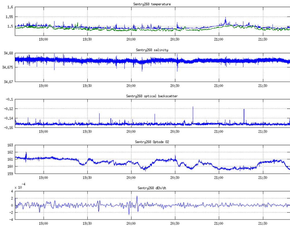
Figure 20: Time series plot of five of the basic sensors on Sentry, from top to bottom, temperature, salinity, optical backscatter, and dissolved Oxygen.
