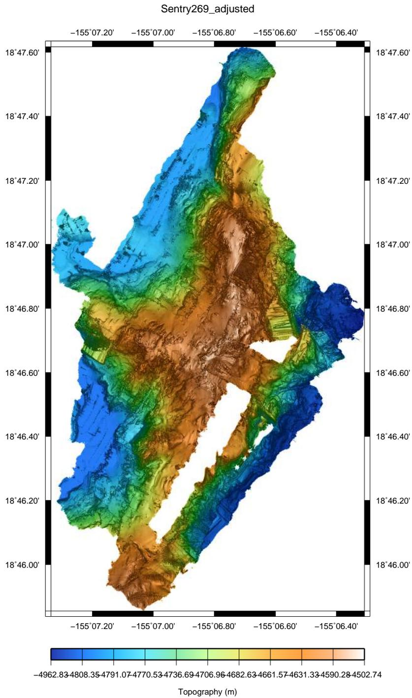
Figure 29: Multibeam bathymetry for dive 269.
