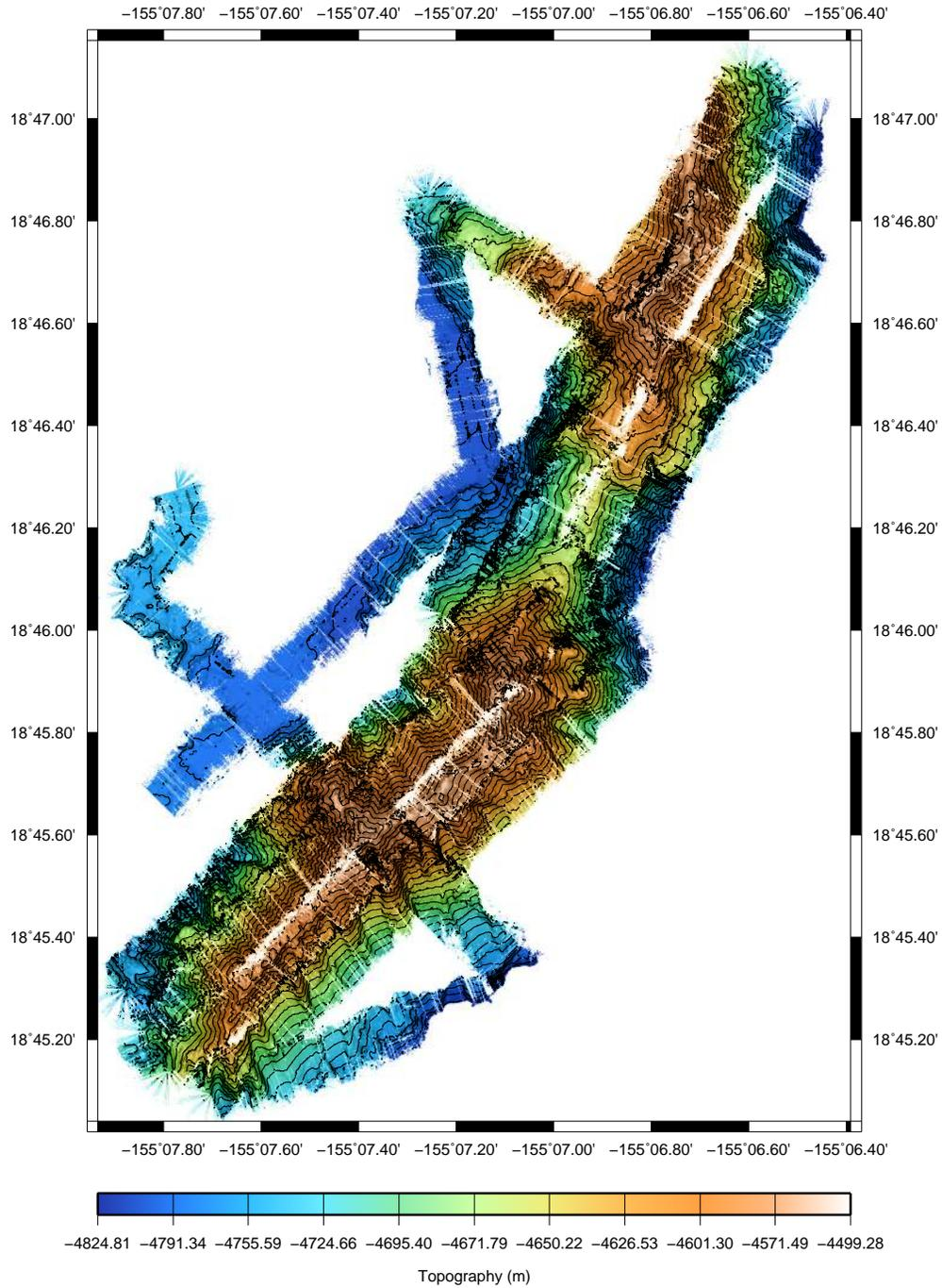
Figure 18: Multibeam bathymetry for dive 266, no adjustment.
