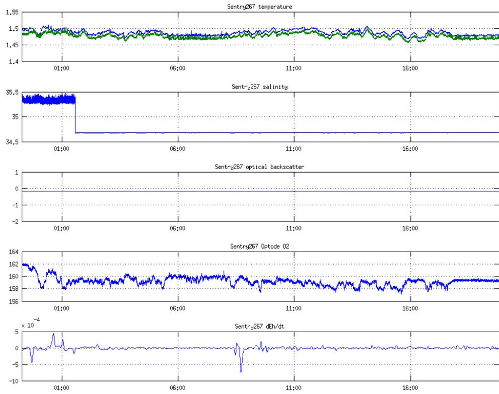
Figure 15: Time series plot of five of the basic sensors on Sentry, from top to bottom, temperature, salinity, optical backscatter, and dissolved Oxygen.
