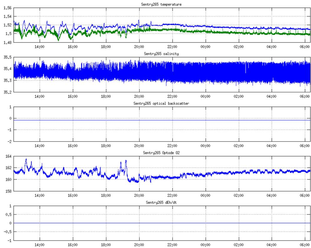
Figure 7: Time series plot of five of the basic sensors on Sentry, from top to bottom, temperature, salinity, optical backscatter, and dissolved Oxygen.
