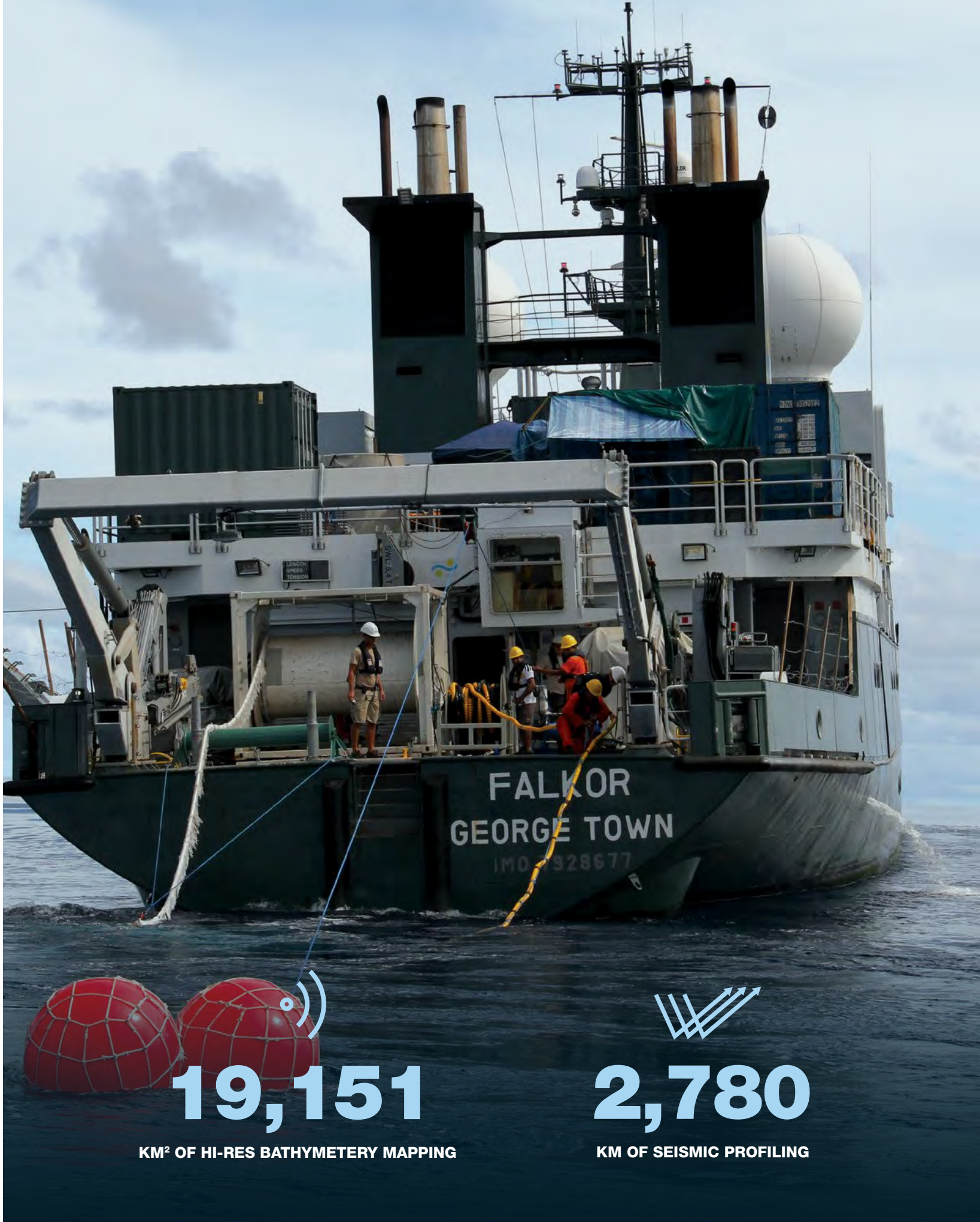
Falkor continues scanning the sea bottom of the Indian Ocean, pulling an air-gun and floats on streamers behind the ship.
